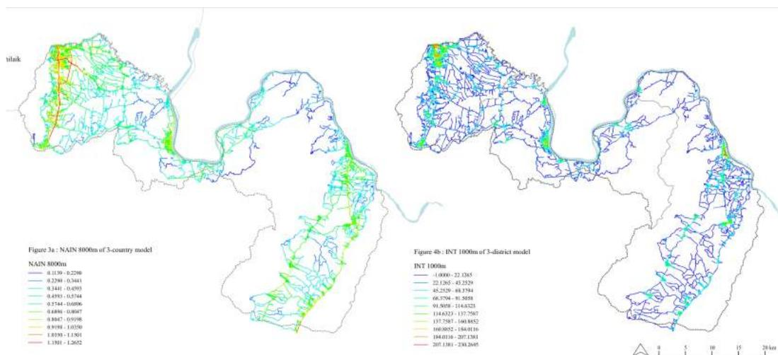
Figure 4: The centrality of angular closeness of the 3-district model: a) NAIN at radius 8,000 metres (8Km); and b) integration at radius 1,000 metres
